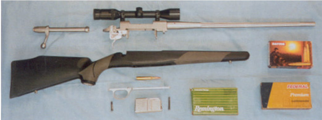
Sako Finnlight disassembled, the wide barrel fluting stands out in this photo.
